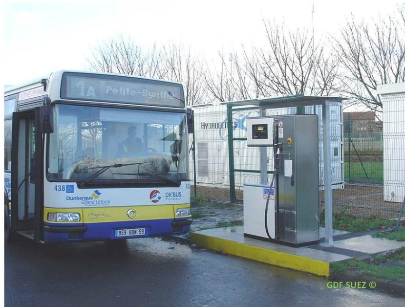
Figure 3 – The Hythane® bus at refuelling.
